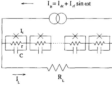
Fig. 1. Schematic circuit of a Josephson junction series array with a resistive load  $R_L$  and external current bias  $I_B$ . Each Josephson junction, with critical current  $I_c$ , is modeled including a shunt resistance  $r$  and a capacitance  $C$ .
