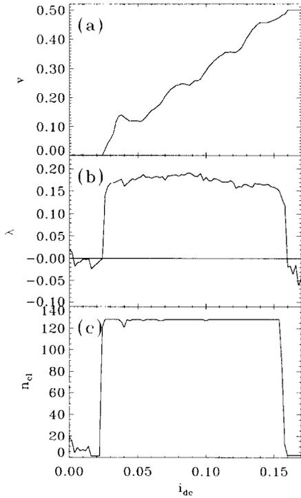
Fig. 2. Behavior of a Josephson junction series array as a function of  $i_{dc}$ . For coupling  $\sigma = 0.4$ ,  $N = 128$  junctions and parameters  $\bar{g} = 0.2$ ,  $\Omega_{rf} = 0.8$ ,  $i_{rf} = 0.61$ . (a) Average voltage  $v$  ( $I$ - $V$  characteristics). (b) Maximum Lyapunov exponent  $\lambda$ . (c) Number of clusters  $n_{cl}$ .
