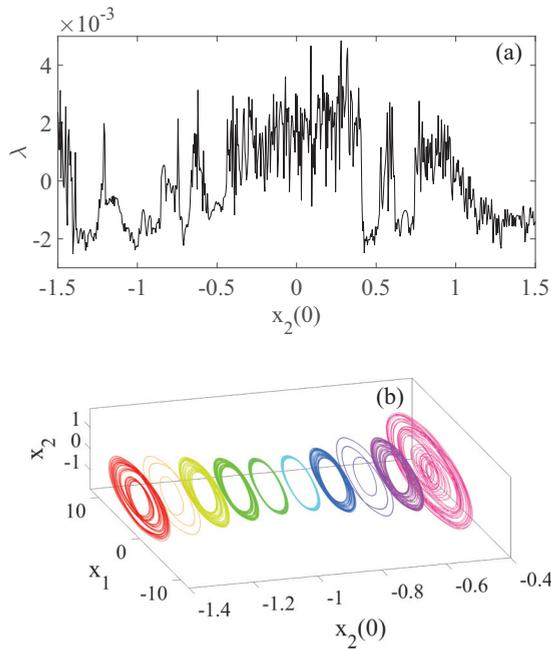
FIG. 4. Largest Lyapunov exponent and the corresponding bifurcation diagram obtained by varying  $x_2(0)$  for a constant value of  $p = 0$  in panels (a) and (b). All other parameters are kept constant at  $x_1(0) = 0$ ,  $e_0 = 1$ ,  $w = 0.2$ ,  $a_1 = 0.21$ ,  $a_2 = 0.001$ ,  $a_3 = 0.2$ , and  $\beta = 0.1$ .
