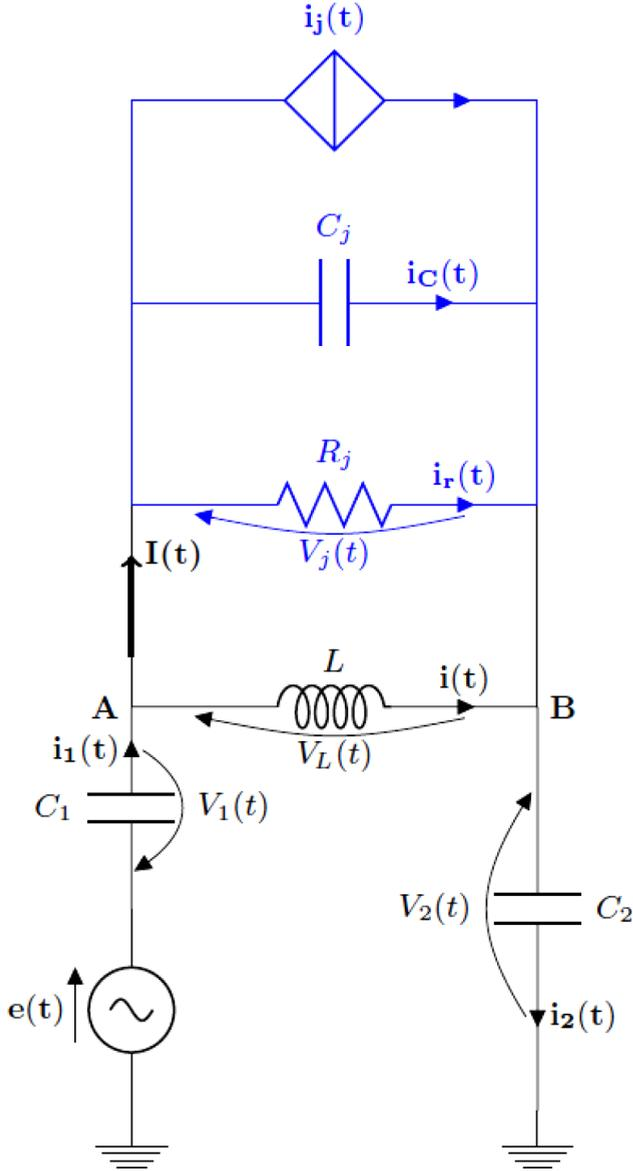
FIG. 1. Schematic diagram of the modified JJ extreme multistable circuit. This circuit is constituted of a Josephson junction element (blue part of the circuit [17,28–31]) connected in parallel to an induction  $L$  which is part of a nonautonomous  $C_1$ - $L$ - $C_2$  resonator. The corresponding labels are defined in the text.
